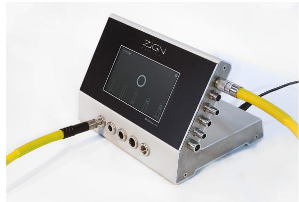
Now the light source adapter can be inserted in the matching light source. Please make sure you select the correct light source. The on-screen images should guide you in the right direction. If you have selected the correct light source, the adapter should have a snug fit which allows for very little room to wiggle inside the light source. Make sure you insert the adapter fully into the light source.
