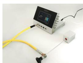
**Insert the scope as far as possible. Rotate lightly while inserting and ejecting. Do not use excessive force, this will damage the interior of the testing probe. Let the scope rest on the table during test (see photo)**
